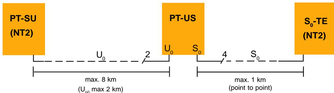
The Interface conversion can be realised as required from  $U_0/U_{p0}$  to  $S_0$  or from  $S_0$  to  $U_0/U_{p0}$  (other Interfaces on request).
