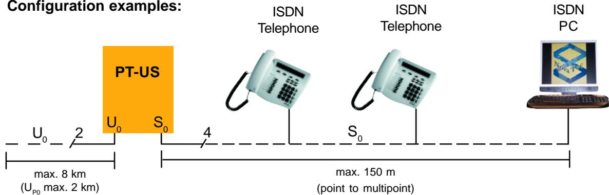
**The PT as an Interface converter:** Converts the two wire  $U_0$  Interface to a four wire  $S_0$  Interface.
