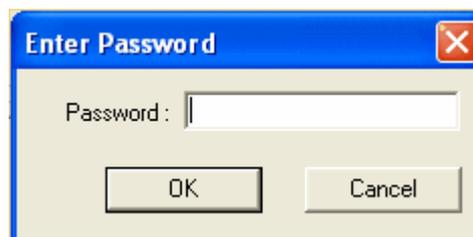
Enter the password and the PIN numbers will be shown un-coded. If you have not changed the password (using the button **Change password...**) the password is **NovaTec**.
