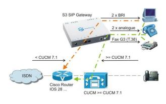
**Example 4:** Connection of BRI, U<sub>p0</sub>- and analogue end devices via the IP net to a PABX
