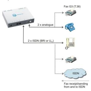
**Example 2:** S3 as RMCS client for the synchronization via ISDN
